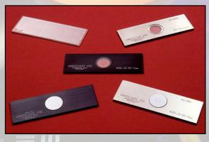
If you require traceable calibration to satisfy NIST or ISO, then you need to have a stage micrometer with a unique engraved serial number. In which case you require our 'PS' series Stage Micrometers. These differ from the 'S' series, because the glass disc is mounted in a stainless steel slide with an engraved, unique serial number. Each slide is supplied in a polished wooden presentation/storage box to distinguish it as a traceable standard of high value.
