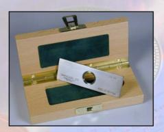
Recent product introductions have included longer scaled micrometers and micrometers with reflective scales for use with top incident lighting rather than transmitted (bottom) light sources.
